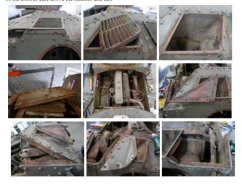
Subsequently, the large fan cover could be released and removed, allowing access to the belt equipment.
