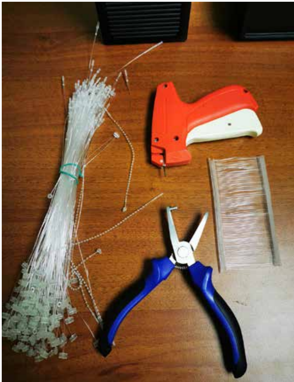
Nylon grips - long or short tying, textile pliers - serve to cover the splint with textile, hole puncher, splints
